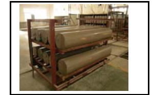
Electrical drying in order to reduce the water content , make the green body suitable for shapping
