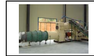
pug mill mud section squeezed into the vacuum chamber ,and get the air out of mud to prepare high performance green body material.
